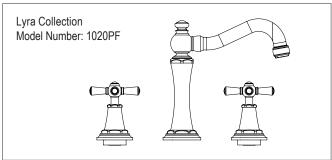
Flush both supply lines before installation, then shut off both supply lines. Minimum hole size for the spout and handle trim is 1-1/4" and maximum of 1-1/2"
