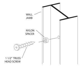
This bath enclosure is equipped with safety teelock wall jambs. When installed properly, the header is permanently locked to the wall jambs and cannot be accidentally dislodged.
