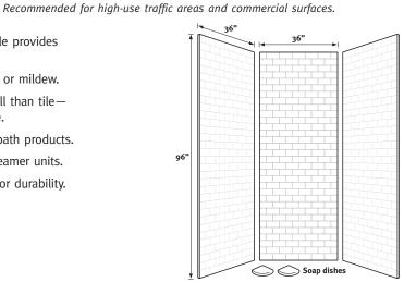
Designed to fit base areas 36" deep or smaller x 36" wide x 96" high or smaller (914 mm x 914 mm x 2438 mm)
