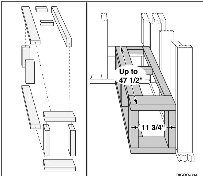
3. In order to eliminate standing water on the bench seat, cut and place three, 2" wide shims on top of each 2 x 4, as shown. Standard shim stock works well for these shims. The shims should be 1/8" thick and taper down to nothing. Also, place a 1/8" thick shim along the wall to completely support the back of the seat.
