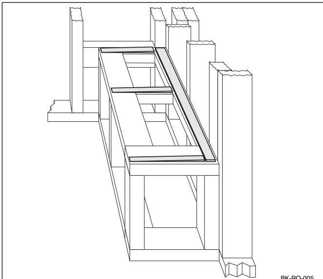
4. Install 1/2" moisture-resistant cement board or greenboard over all the surfaces of the seat area (1, 2, & 3). Follow the wall board manufacturer's recommendations for installation.
