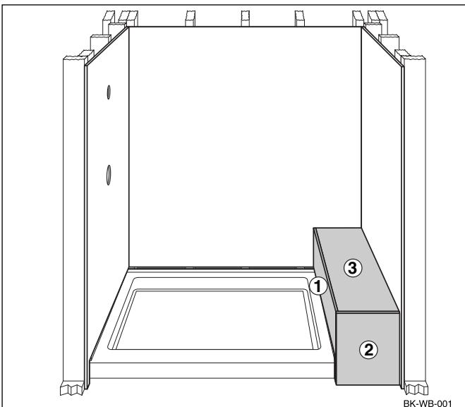
5. Apply a coat of water or oil-based primer/sealer to all the surfaces of the cementboard or greenboard (follow the manufacturer's instructions). Allow the primer to dry thoroughly before applying any clear silicone.
