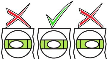
**! Leveling the floor is critical for a properly aligned installation. Thinset can be used to level floor. Be careful not to block the drain hole position.**
