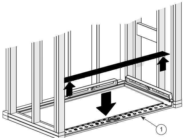
**B.** Install drain on base as per drain installation instructions.
