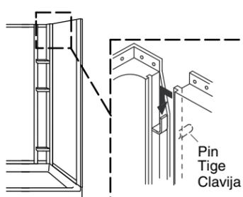
**16** The front edges should be flush, with no more than a 1/32" (1 mm) gap.
