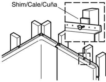
**19** Cover the framing with water-resistant wallboard. Install the finished wall material.
