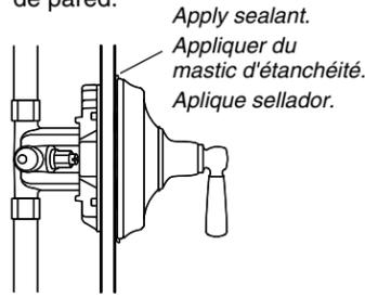
**21** After painting, apply 100% silicone sealant where the unit contacts the finished wall.
