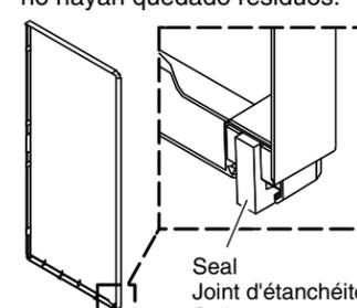
**15** Install the end walls. Engage the end wall pins in the back wall slots.
