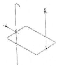
24. First slip the wall tee onto the shower riser about 10" below the crook in the riser. Only tighten slightly as later an adjustment will most likely be necessary. Connect portions of the riser with the union nut.
