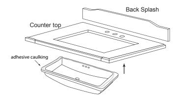
**Step 1:** Apply adhesive caulking around the topside of rim near the edge, Carefully raise sink in place, align, and press firmly
