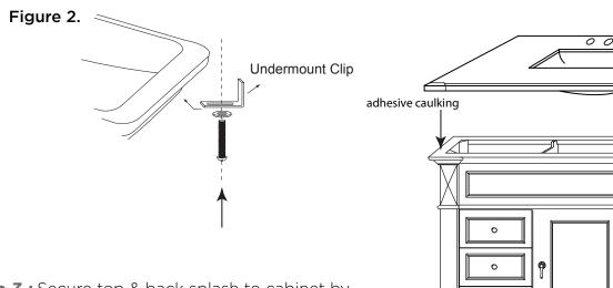
**Step 3 :** Secure top & back splash to cabinet by using adhesive caulk
