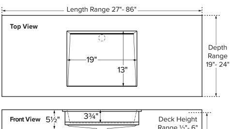
**NOTE:** Counter-sinks with a length of 36" and under have a maximum depth of 23".
