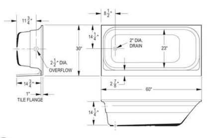
**General:** Furnish and install as shown on plans, TOPAZ<sup>®</sup> bathtub as manufactured by E.L. Mustee & Sons, Inc. Shall be a fiberglass 30" x 60: right hand or left hand Model \_\_\_\_\_\_. Construction shall be molded, reinforced fiberglass using matched metal molds under extreme heat and pressure. Shall meet ANSI Specification Z 124-2011. Color: \_\_\_\_\_\_ (White, Bone, Biscuit) Weight: 74 lbs. Install in compliance with local codes.
