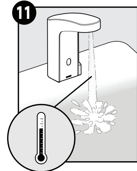
If temperature is over (>) 120°F (49°C) go to 7. If less(<) 120°F (49°C), turn off system.
