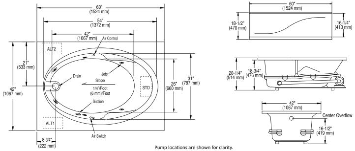
STD - standard pump location. ALT1 and ALT2 - alternate pump locations are optional.
