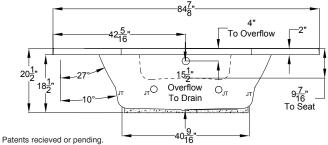
Drop-in-Hole Size: Operating Capacity: Overflow Capacity: Floor Loading / sq.ft.: Carton Weight: Cube: See Diagram 58 Gal. 76 Gal. 44.1 lbs. 127 lbs. 50.9 ft.<sup>3</sup>
