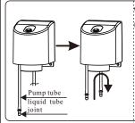
When the pump tube is blocked or adhered, refer to the following steps to clean the tube.
