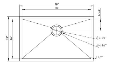
Dimensions of fixture are nominal and may vary within the range of tolerances established by ANSI Standard A112.19.2. Dimensions and specifications subject to change without notice.
