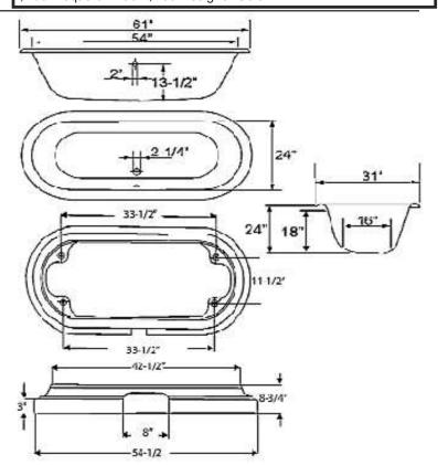
Dimensions of fixture are nominal and may vary within the range of tolerances established by ANSI Standard A112.19.2. Dimensions and specifications subject to change without notice.
