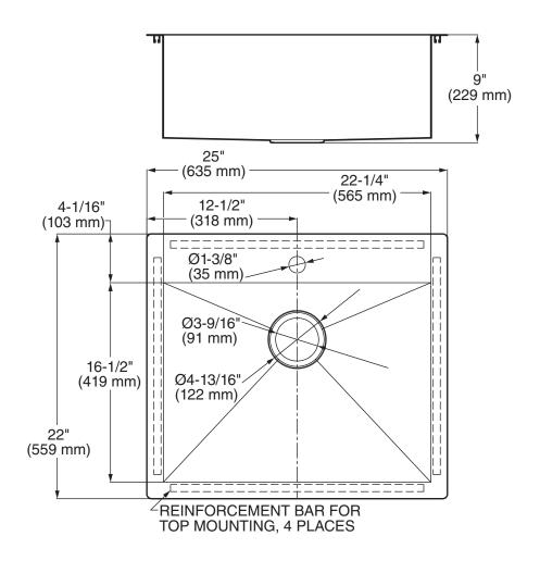
**NOTES:**\* DIMENSIONS SHOWN FOR LOCATION OF SUPPLIED AND "P" TRAP ARE SUGGESTED. FITTINGS NOT INCLUDED WITH FIXTURE AND MUST BE ORDERED SEPARATELY. SEALING COMPOUND SUPPLIED BY OTHERS.
