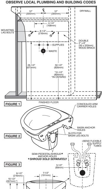
Top of front rim must be mounted at less than 864mm (34") from the finished floor to meet ADA and ANSI A117.1 requirements. In Ontario, the code requires a height of 838mm (33"). Check local codes.
