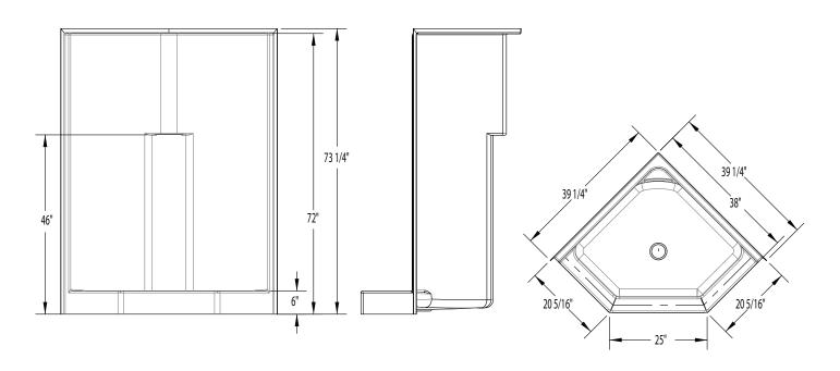
FEATURES Ibs Dimensional Tolerance ± %". Dimensions needed for site preparation should be measured from the unit. Aquatic assumes no responsibility for preparatory work.
