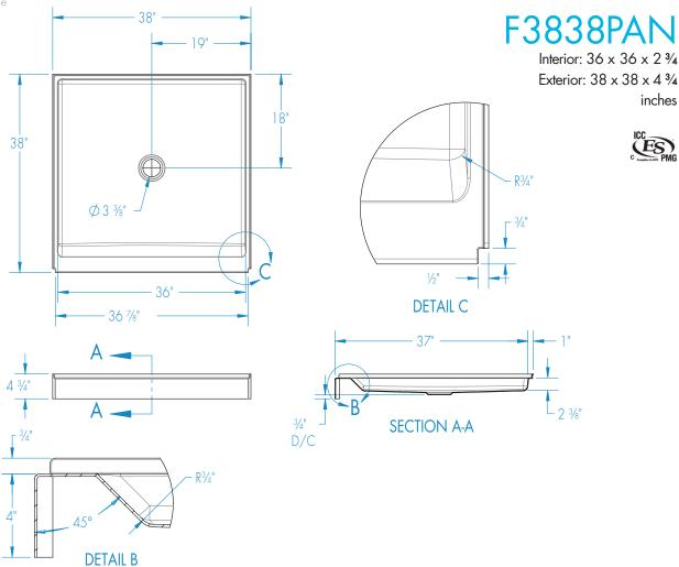
FEATURES Dimensional Tolerance ± %". Dimensions needed for site preparation should be measured from the unit. Aquatic assumes no responsibility for preparatory work.
