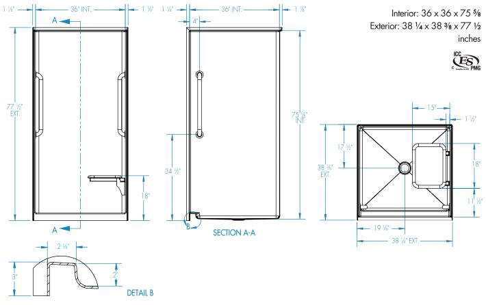
FEATURES Dimensional Tolerance ± %". Dimensions needed for site preparation should be measured from the unit. Aquatic assumes no responsibility for preparatory work.
